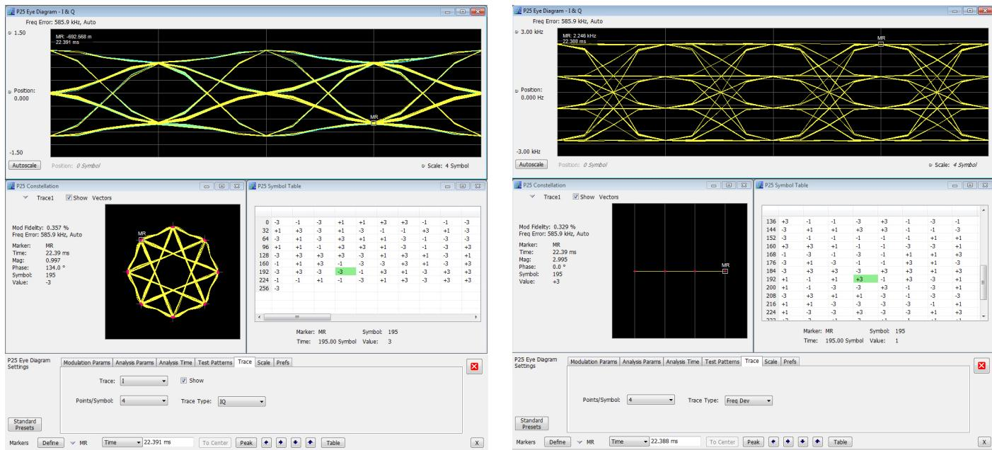
Figure 12. Correlated Markers in Eye Diagram, Constellation Diagram, and Symbol Table for H-DQPSK. The left screen shot shows the IQ traces, whereas the right screen shot shows the frequency deviation trace for the same H-DQPSK signal.
