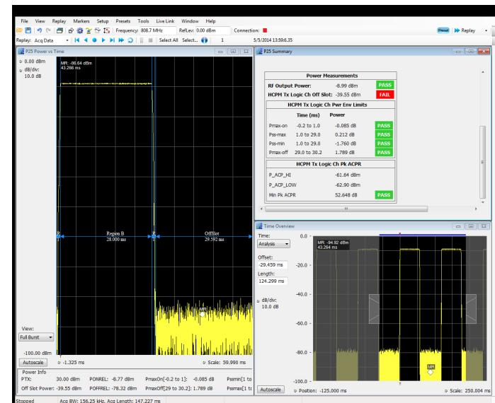
Figure 23. H-CPM Two-Slot TDMA timing diagram and logical channel peak ACPR measurement.
