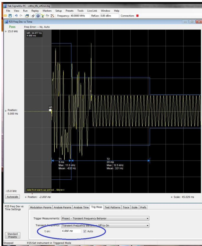
Figure 20. Transient Frequency Behavior measurement control.
