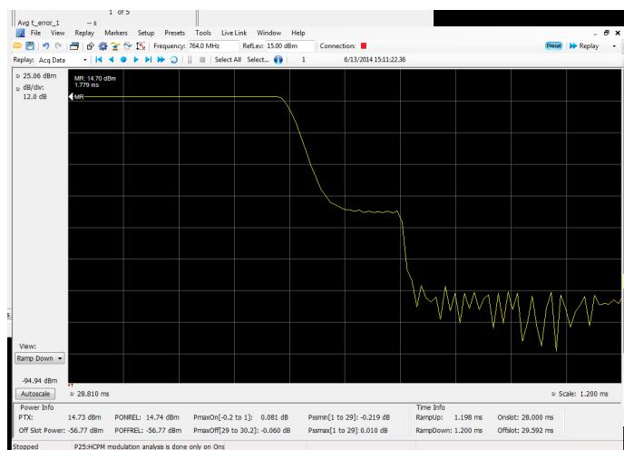
Figure 25. H-CPM TDMA transmitter power envelope ramp down trace shown in P25 Power vs. Time display and all power envelope measurements in P25 Summary.
