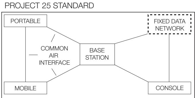
**Figure 1.** P25 Common Air Interface.
