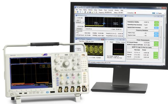
**Figure 4.** MDO4000B with SignalVu-PC running P25 analysis software (opt. SV26).
